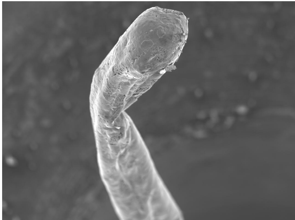
Figure-3: SEM photo of 4% 0,25mm nickel plated copper wire after 5 minutes exposure at 1100°C
